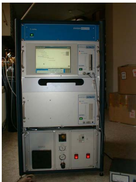
Complete installation for an ozone precursor instrument, two gaschromatographs, including gas supply
