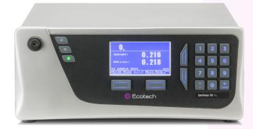
The Serinus® 10 Ozone  $(O_3)$  analyser delivers precise and reliable performance at excellent value. It uses proven non-dispersive ultraviolet (UV) absorption technology to measure  $O_3$  in ambient air (LDL < 0.5 ppb, range 0 to 20 ppm).
