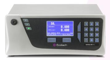
The Serinus<sup>®</sup> 50 sulfur dioxide  $(SO_2)$ analyser delivers precise and reliable performance at excellent value. It uses proven pulsed UV fluorescent radiation technology to measure  $SO_2$  in ambient air (LDL < 0.3 ppb, range 0 to 20 ppm).
