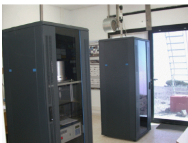
MicroPNS HVS sampler for 19" rackmount version and sampling heads outside roof
